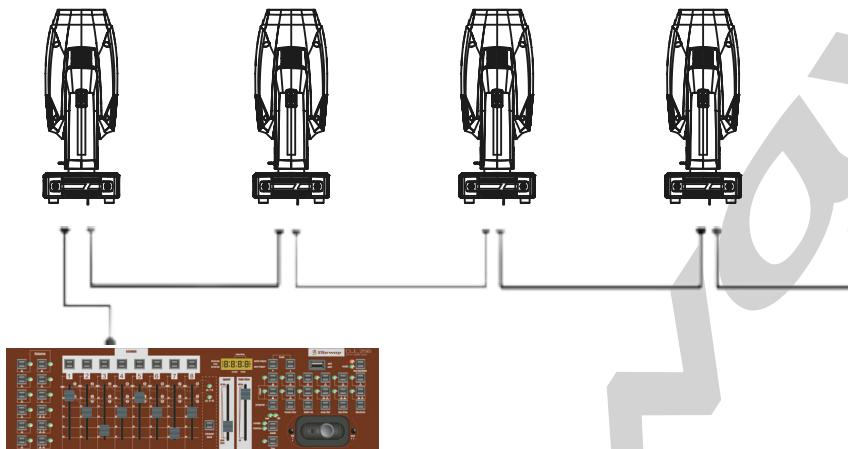
The projectors are connected in series to a DMX console.
